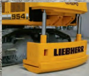
**Counterweight can be hydraulically lowered** for lowering the weight during transport
