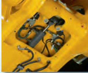
**Piston rod protection for boom cylinders**
