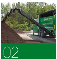
The fine particles are discharged by a onepiece corrugated edge belt.
