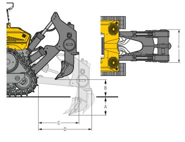
\* Best performance to operate in loose material – deep shanks are designed for light and moderate duty
